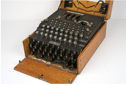
An Enigma I machine. The plugboard can be seen on the front of the machine. The keyboard and lampboard are located on top of the machine. Above the lampboard are three little windows, through which one can see the current configuration of the rotors.
