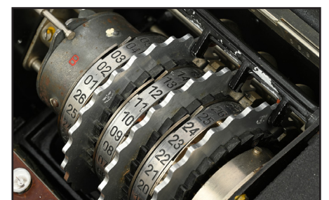
A closeup of the rotors of the Enigma machine. Sometimes the numbers 01-26 would be used instead of the letters A-Z.
